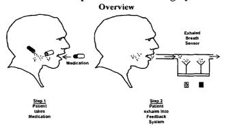
PCMS includes marker compound included in medication that is exhaled into detection system for accurate and reliable monitoring off-site
